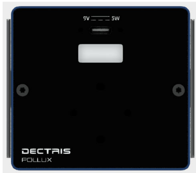
Figure 4. The POLLUX Panorama detector (back view). The back of the detector head features the USB-C data port for the connection to the detector control system (DCS).
