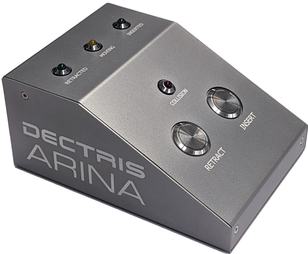
Figure 4.4: The DECTRIS ARINA® Control User Interface Box
