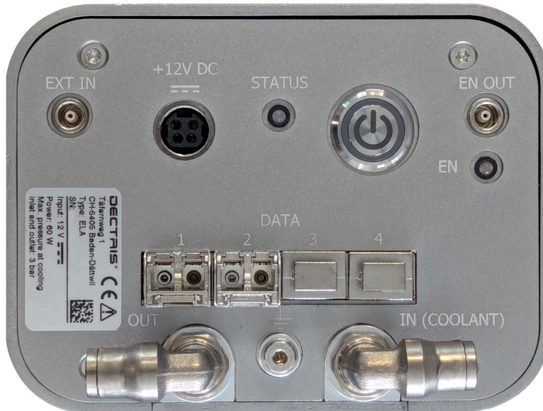
Figure 4.3: The DECTRIS ELA® Detector (back view)
