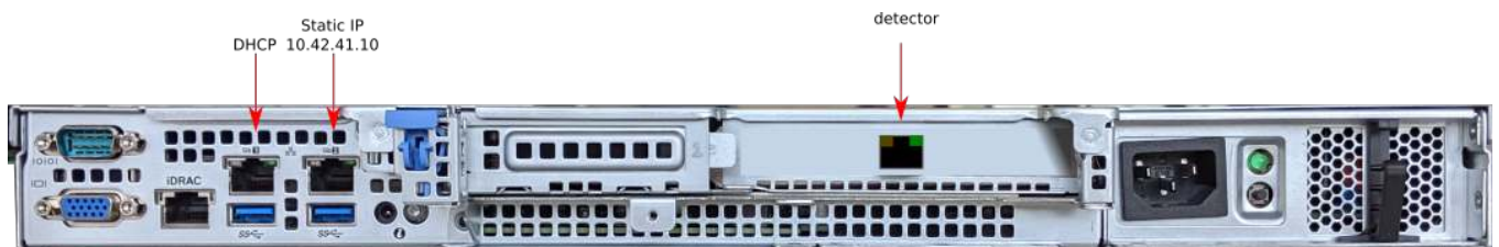
Figure 4.6: EIGER R 1M detector control unit as seen from the back. Back view of detector control unit with network interfaces.
